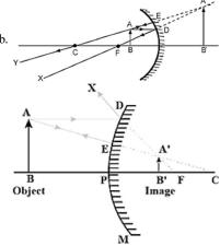
c. Concave mirrors can also be used to obtain a magnified and real image of an object. When an object is placed anywherebetween infinity to focus we get a real and magnified image.
