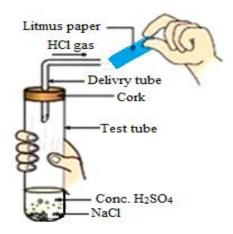
Blue litmus paper is brought near the mouth of the delivery tube to check the presence of hydrochloric acid but no change is observed in the colour of litmus paper because:
